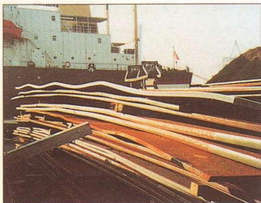
Plates. Mechanical damage clause (top plate in stack): edges waved along entire length.
