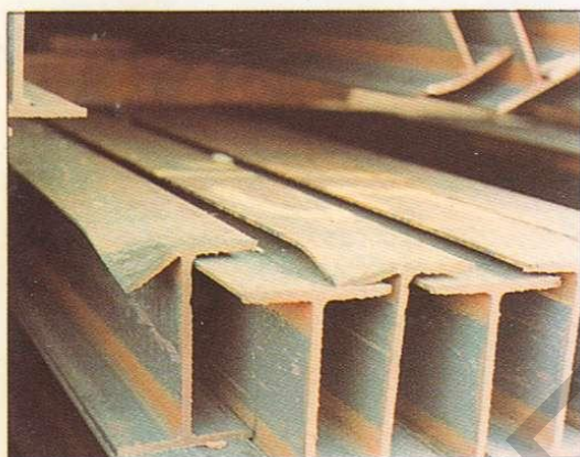
Nest of beams. Mechanical damage clause (left hand beam): flange bent in one position at end.
