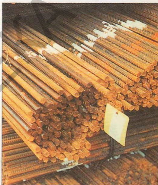
Reinforcing bars in bundles with dampness evident. Surface condition clause: rust stained, wet before shipment .
