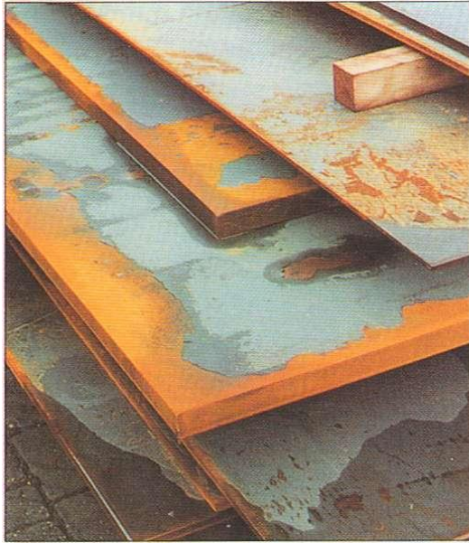
Plates with most mill scale, but handling has also fragmented mill scale from edges. Surface condition clause: partly rust stained, wet before shipment.
