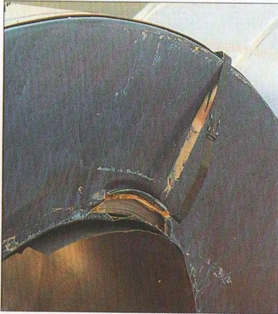
Wrapped coil damaged by forklift. Mechanical damage clause: packing torn open in one place at inner circumference. Visible cargo is scored. Affects 15 windings.
