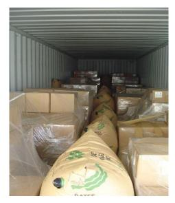
Make sure that the weight of your load is evenly distributed in length and width, of the container or truck. Take special care with the reels, such as for example steel rolls, which with their displacement may cause damage to the container or the truck. For these cases it is highly recommended to use *cargo airbags*.
