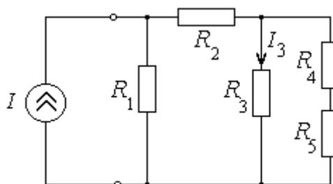
$$R_1 = 2 \text{ кОм}, R_2 = 1 \text{ кОм}, R_3 = 3 \text{ кОм}, R_4 = 1 \text{ кОм}, R_5 = 4 \text{ кОм}, I = 3,9 \text{ мА}.$$
