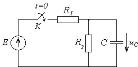
$$R_1 = 200 \text{ Ом}, R_2 = 600 \text{ Ом}, C = 40 \text{ мкФ}, E = 1 \text{ В}.$$
