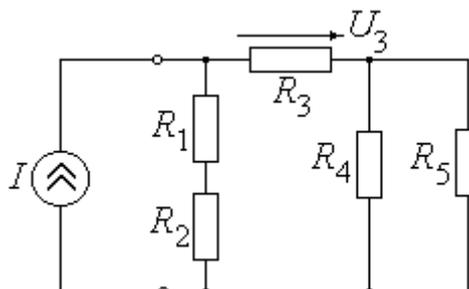
$$R_1 = 500 \text{ Ом}; R_2 = 500 \text{ Ом}; R_3 = 2 \text{ кОм}; R_4 = 2 \text{ кОм}; R_5 = 2 \text{ кОм}; I = 10 \text{ мА}.$$
