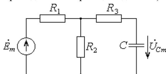
$$R_1 = 10 \text{ Ом}, R_2 = 20 \text{ Ом}, R_3 = 30 \text{ Ом}, \omega = 10^5 \text{ рад/с}, C = 50 \text{ нФ}, \dot{E}_m = 6,1 \cdot \exp(j \cdot 0^\circ) \text{ В}.$$
