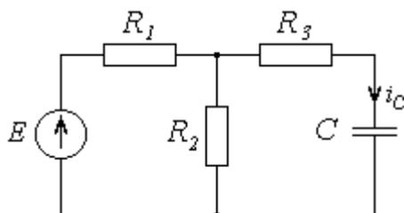
$$R_1 = 1 \text{ кОм}, R_2 = 1 \text{ кОм}, R_3 = 500 \text{ Ом}, C = 0,25 \text{ мкФ}.$$
