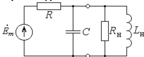
$$R = 200 \text{ Ом}, C = 50 \text{ нФ}, R_n = 50 \text{ Ом}, L_n = 2 \text{ мГн}, \omega = 10^5 \text{ рад/с}, E_m = 20 \text{ В}.$$
