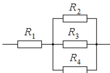
$$R_1 = 1 \text{ кОм}, R_2 = 4 \text{ кОм}, R_3 = 4 \text{ кОм}, R_4 = 2 \text{ кОм}$$
