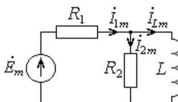
$$R_1 = 126 \text{ Ом}, R_2 = 70 \text{ Ом}, \omega = 6 \cdot 10^4 \text{ рад/с}, L = 400 \text{ мкГн}, \dot{E}_m = 5 \cdot \exp(-j \cdot 30^\circ) \text{ В}.$$
