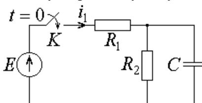
$$R_1 = 100 \text{ Ом}, R_2 = 400 \text{ Ом}, C = 50 \text{ мкФ}, E = 5 \text{ В}.$$
